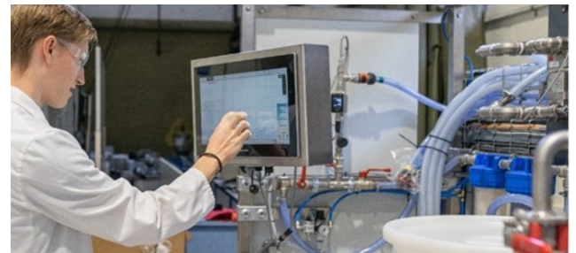
Figure 2. operating the pilot plant to process the fermented lactic acid mixture
